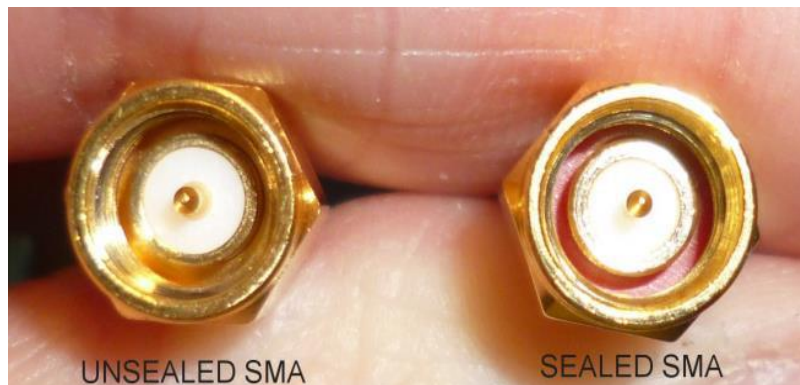
Figure 4: Unsealed and Sealed SMA Connectors
