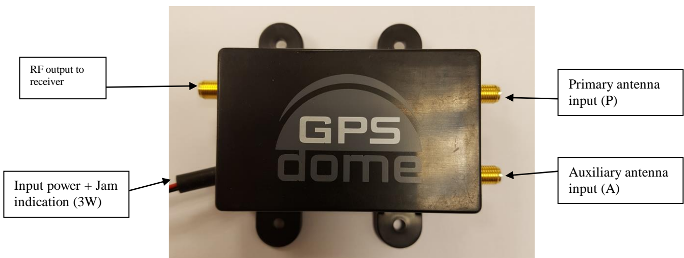
Figure 1b: GPS Dome 1.01-DF – General view
