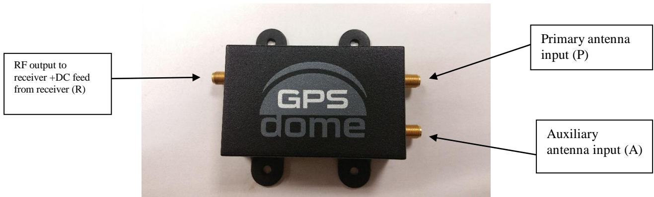
Figure 1a: GPS Dome 1.01 – General view
